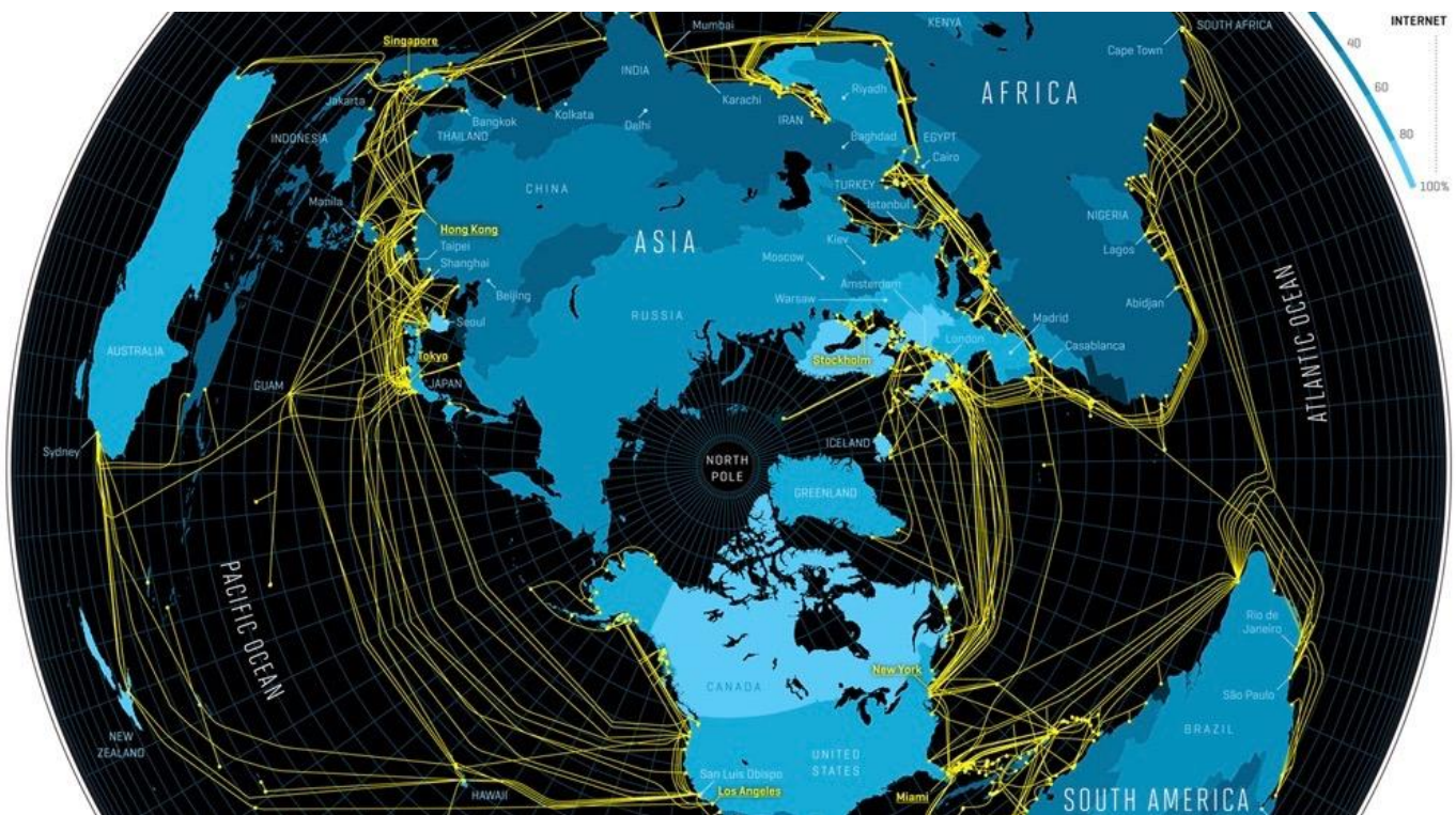
major global submarine fiber-optic lines. Image: GeoTel Communications and Nicolas Rapp/Fortune magazine
